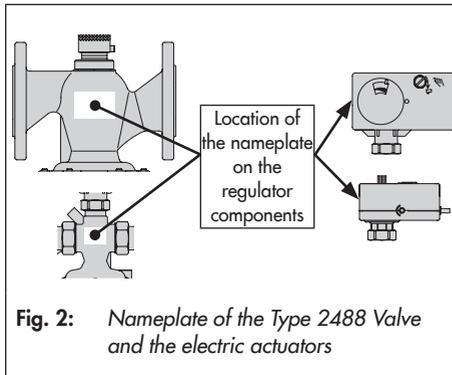
**Fig. 2:** Nameplate of the Type 2488 Valve and the electric actuators
