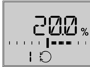
Fig. 43: Start screen with PID controller application (PID) · Displayed reading: process variable
